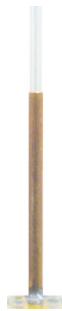
Fig. 2. Monopole antenna: coaxial cable with the outer metal conductor stripped from the termination. The region free from the shield acts as an active zone (transmitting zone), as it couples with the surrounding medium.
